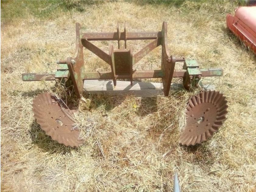
*Moulder, attaches to three-point linkage on tractors*
