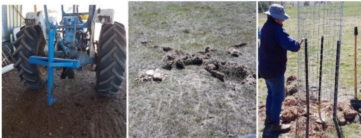
*The single tyne ripper can be used to prepare ground for single paddock trees, as well as for longer strips.
