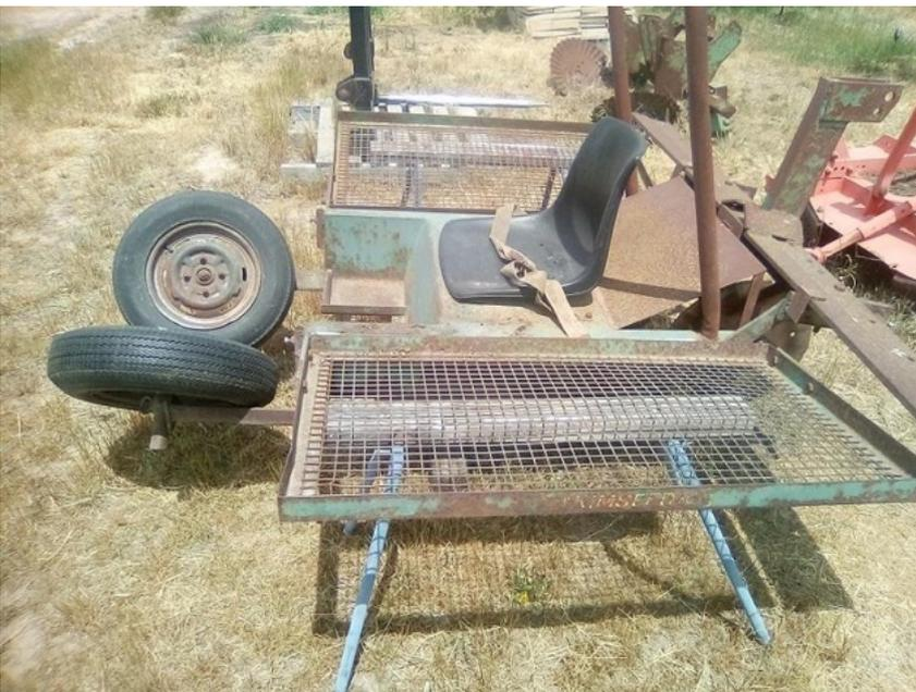
*Tractor drawn tree planter, attaches to three-point linkage on tractors*
